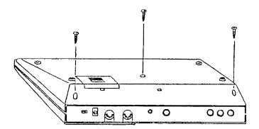
2. Separate the two halves of the case. Unplug the 3x Molex connectors joining the top case to the bottom, as well as the connector from the battery box. Remove the 2x screws which secure the main board to the bottom case and lift it out of the case.
