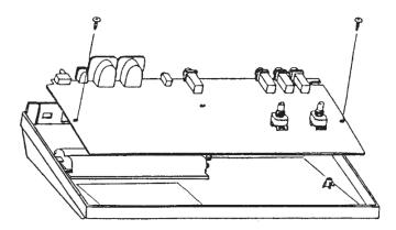
3. Locate IC11 on the main board and desolder it, being careful to not lift any pads. In its place, solder the included IC socket. The original Roland chip is no longer needed, but you might want to keep it somewhere safe.
