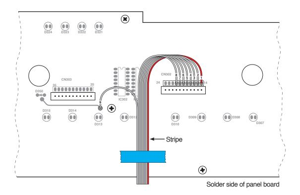
12. Reinstall the main PCB assembly in the top case, reconnecting the two cables that join it to the panel board. Like the disassembly, this is easiest done with the machine on end.
